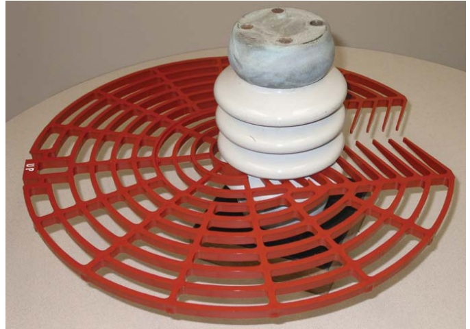
Figure 2: Improper Fit, Small Inner-Ring Diameter.
