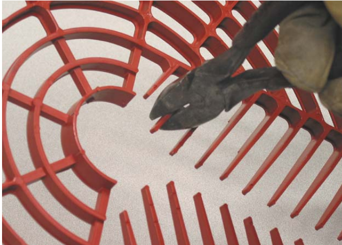
Figure 5: Trimming Flexible Fingers.
